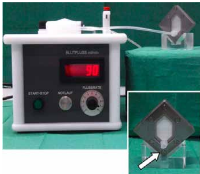
Fig. 1: Flow chamber setup for the exposure of endothelialised hollow fibre membranes to flow conditions.
